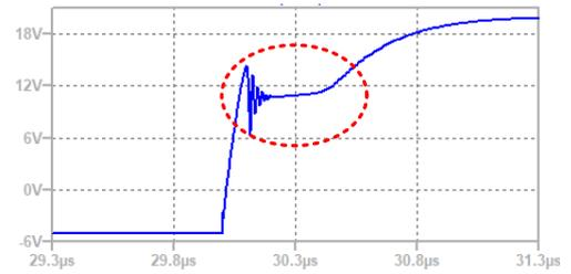
Fig. 7. Simulation waveform of the gate voltage during turn-on transient.
