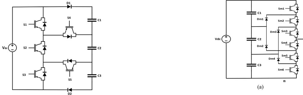
FIGURE 2. Proposed voltage balancing converter.
