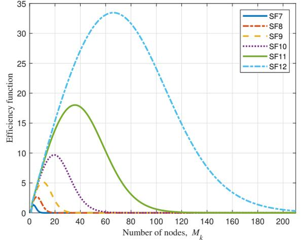
Fig. 5. The efficiency function versus the number of LoRaWAN nodes for different SFs
