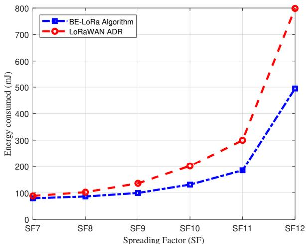
Fig. 9. Energy consumption comparison between BE-LoRa and LoRaWAN ADR
