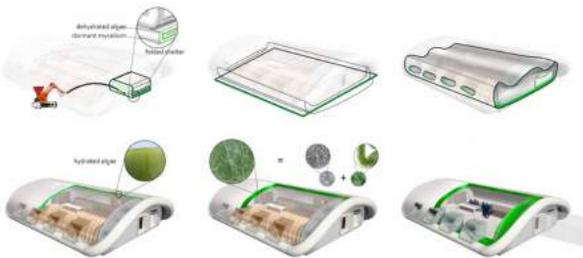
Fig. 11. Fully encased structures self-assemble when water, CO<sub>2</sub>, and heat are added by a robot (image credit: rehouse studio)
