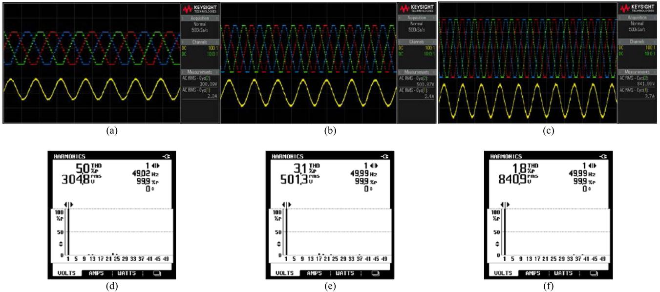
**FIGURE 13.** Experimental results at  $m = 1$  and  $f = 50\text{Hz}$  for: (a) line voltages and current of 1<sup>st</sup> case study, (b) line voltages and current of 2<sup>nd</sup> case study, (c) line voltages and current of 3<sup>rd</sup> case study, (d) harmonic spectrum of 1<sup>st</sup> case study, (e) harmonic spectrum of 2<sup>nd</sup> case study, (f) harmonic spectrum of 3<sup>rd</sup> case study.
