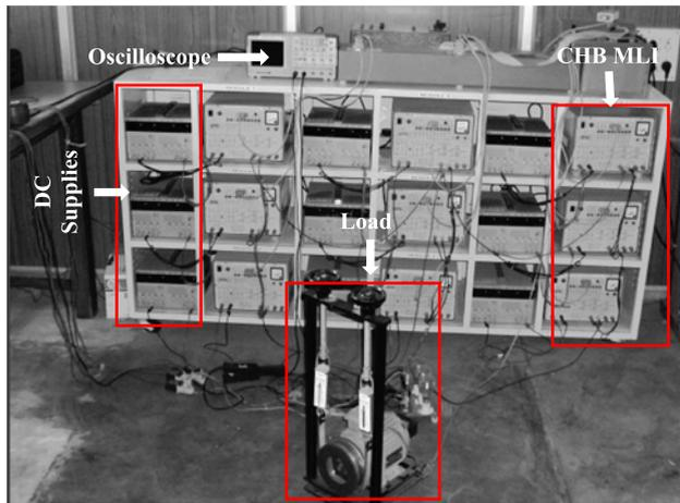
FIGURE 12. Experimental setup for the three-phase CHB MLI.
