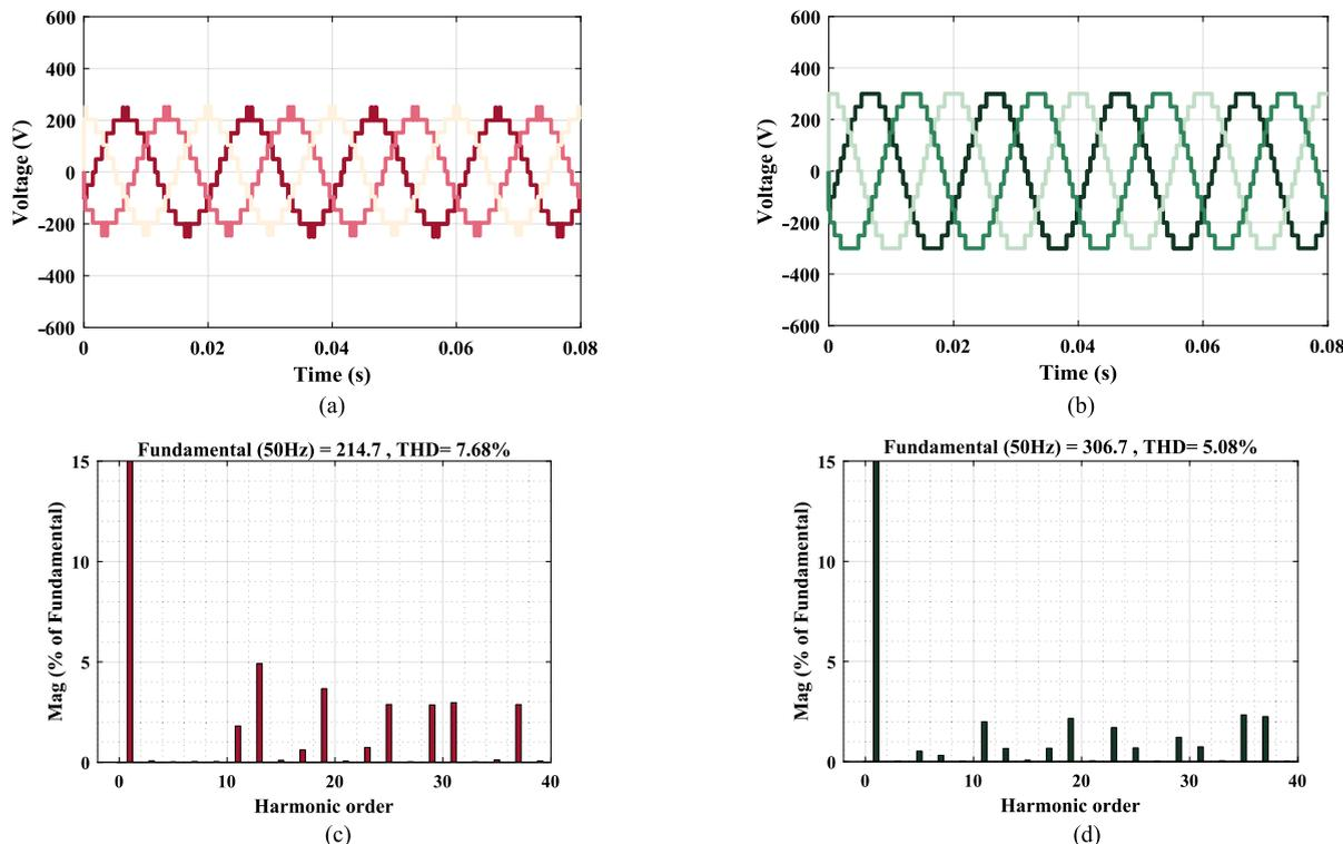
FIGURE 6. Simulation results of three-phase 7-level CHB MLI: (a) line voltages at  $m = 0.6$ , (b) line voltages at  $m = 1$ , (c) harmonic spectrum of line voltage ab at  $m = 0.6$ , (d) harmonic spectrum of line voltage ab at  $m = 1$ .
