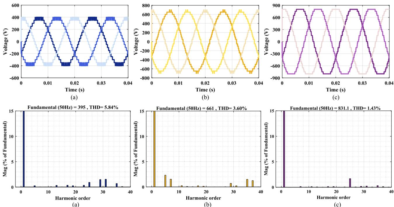
**FIGURE 10.** Simulation results of three-phase 17-level CHB MLI: (a) line voltages at  $m = 0.4$ , (b) line voltages at  $m = 0.7$ , (c) line voltages at  $m = 1$ , (d) THD of line voltage ab at  $m = 0.4$ , (e) THD of line voltage ab at  $m = 0.7$ , and (f) THD of line voltage ab at  $m = 1$ .
