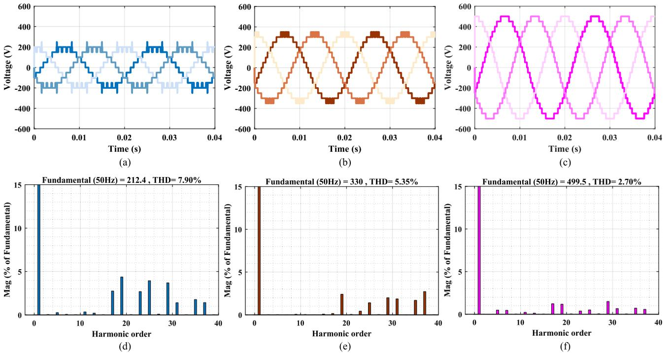
FIGURE 8. Simulation results of three-phase 11-level CHB MLI: (a) line voltages at  $m = 0.3$ , (b) line voltages at  $m = 0.6$ , (c) line voltages at  $m = 1$ , (d) THD of line voltage ab at  $m = 0.3$ , (e) THD of line voltage ab at  $m = 0.6$ , and (f) THD of line voltage ab at  $m = 1$ .
