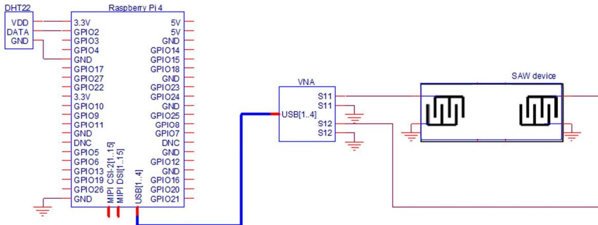
Figure 2 Circuit diagram of Raspberry Pi pinout and SAW control
