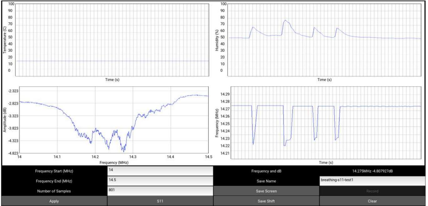
Figure 3 GUI used to monitor SAW device and DHT22
