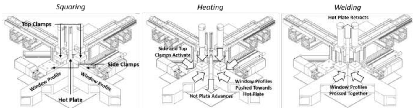
**Figure 1.** Automated hot plate welding process illustration.
