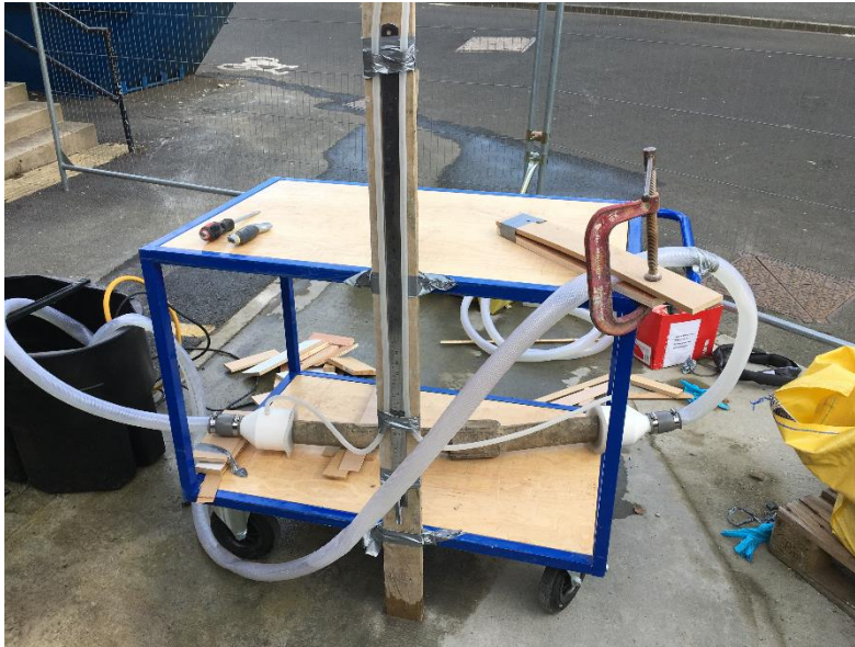
Figure 6: Overview of the experimental rig showing the jointed pipe under test, with manometer and flow control. To the left is the sump tank in which the pump was located
