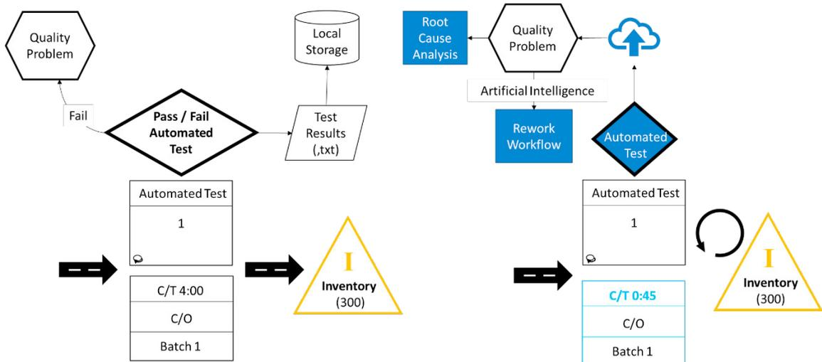
Fig. 3. Product test evaluation. *Left*: current state. *Right*: forecasted future state with stepwise upgrade to Industry 4.0.
