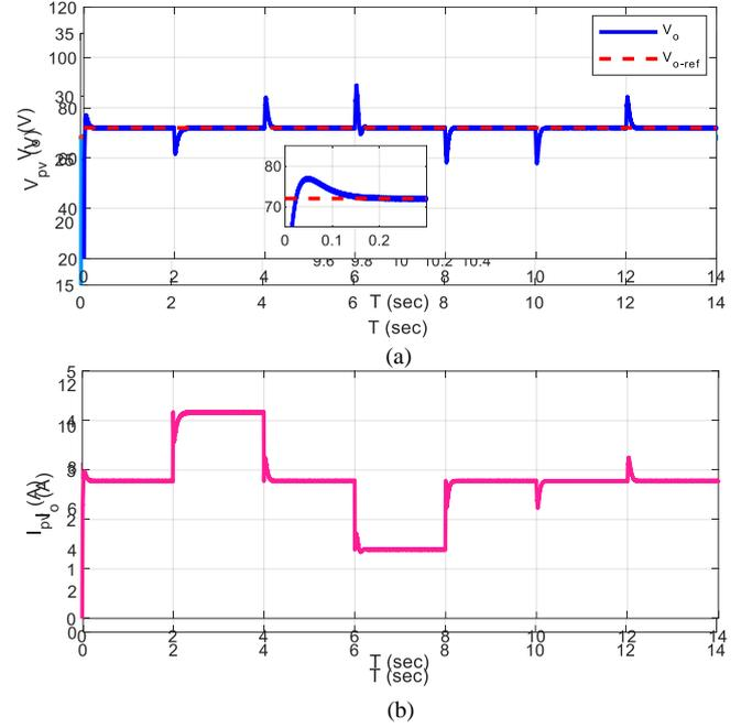
Fig. 4. Results of MPPT control. (a) PV output voltage, (b) PV output current
