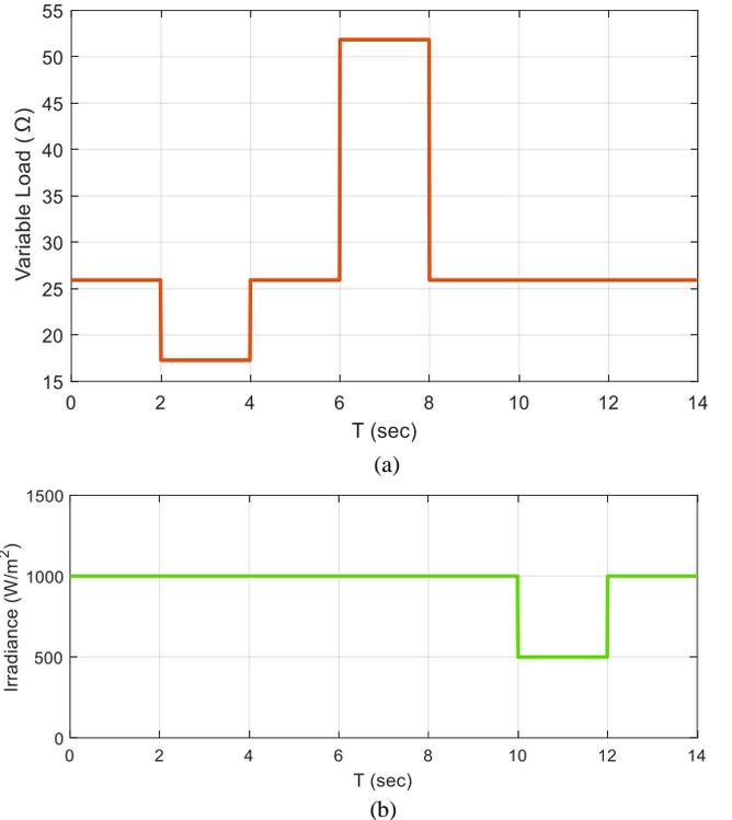
Fig. 5. Case studies. (a) Variable load profile, (b) Solar irradiance change
