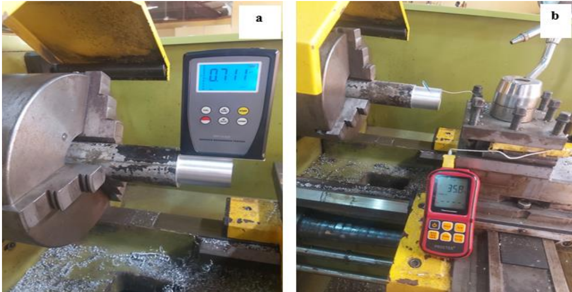
Fig. 3. (a) Surface roughness tester (SRT -6100) taking readings on the sample (b) Cutting temperature tester (Dual Channel Thermocouple Thermometer)
