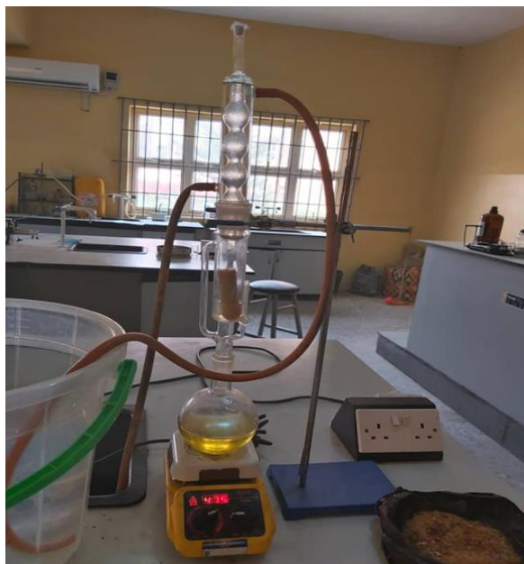
Fig. 2. Extraction process of African star seed oil using Soxhlet extractor with n-Hexane
