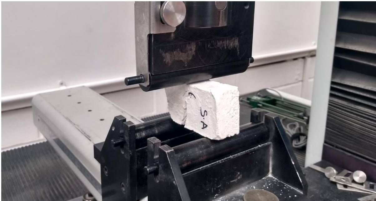
Figure 6 - Set-up of the three-point bending test and typical failure mode of a paste specimen.
